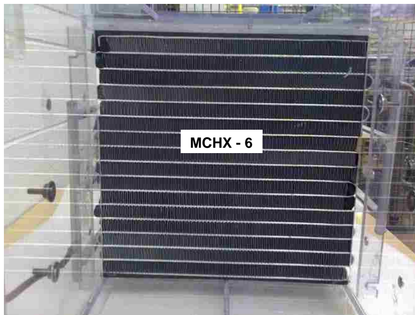
Figure B2.6d. Photograph of fabricated microchannel prototype design in current study– MCHX-6
