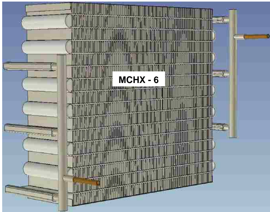
Figure B2.6c. Solid model of fabricated microchannel prototype design in current study– MCHX-6
