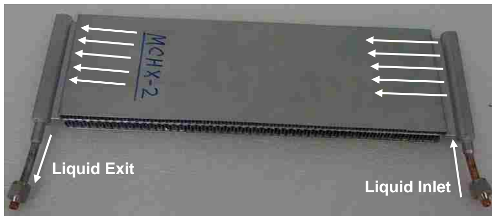
Figure B2.2c. Photograph of current fabricated multi-port microchannel test specimen – MCHX-2
