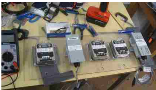
q. Airside Pressure Transducers Panel Making
