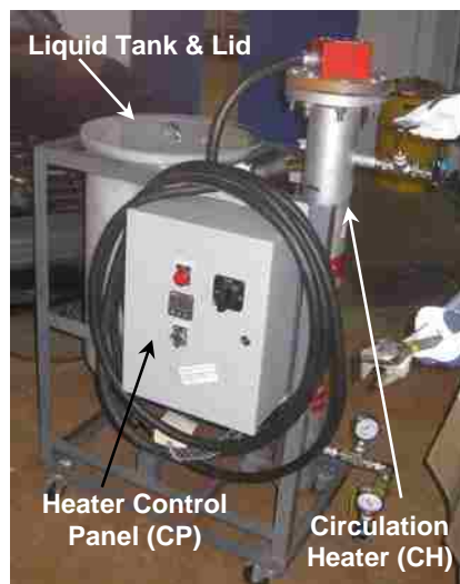
k. Tank-Heater Cart Unit Assembly & Fitting
