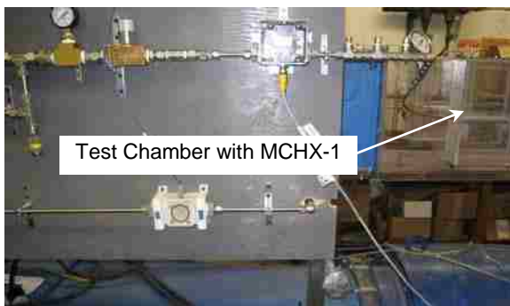
i. Liquid handling system panel construction-5
