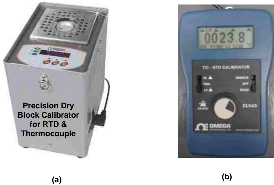
Figure 4.15. (a) Precision thermocouple and RTD calibrator (Dry block) and (b) Highly accurate handheld digital dual thermocouple-RTD calibrator used in current study.
