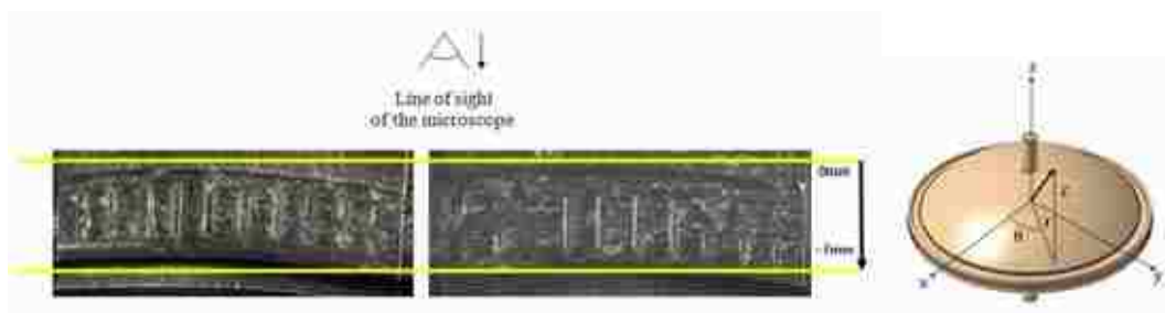
Figure 22: Line of sight for the microscope. (Perpendicular to the center axis, z, of the assembly)
