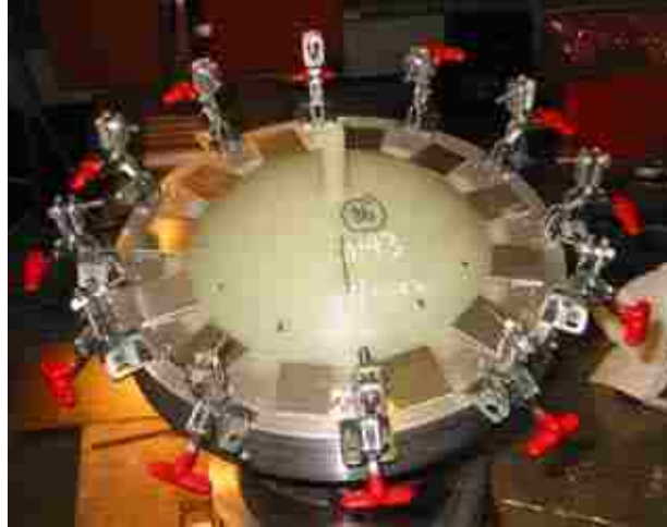
Figure 25: Shields used for burst tested samples
