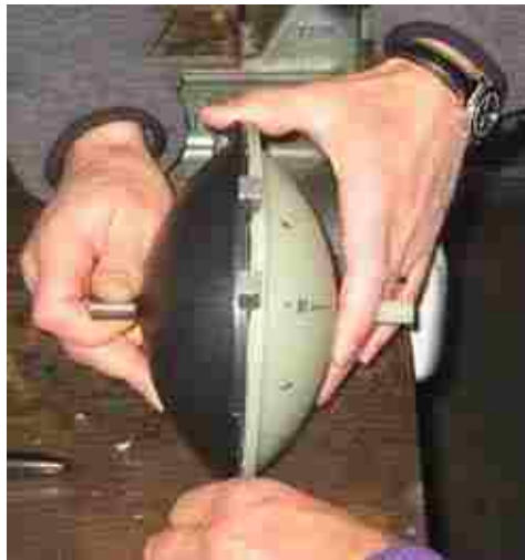
Figure 24: Welded sample being separated for fracture surface analysis. Wedges are inserted between the welded inserts to “pry” apart the components. The clamps’ shadow prevented the laser beam from reaching the part between the inserts, thus these areas are not welded.
