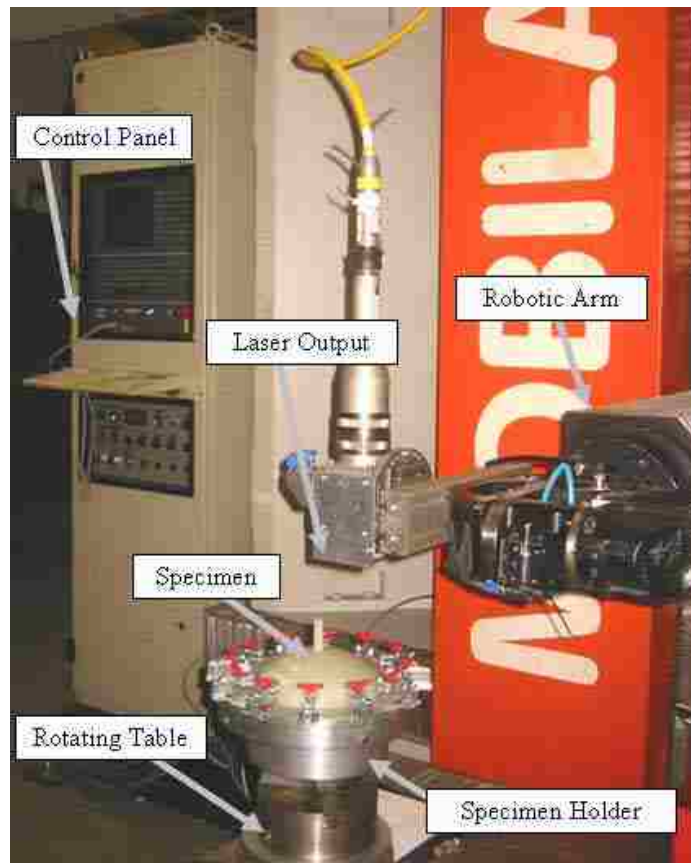
Figure 20: Equipment setup for the Nd:YAG laser at Fraunhofer Center for Laser Technology
