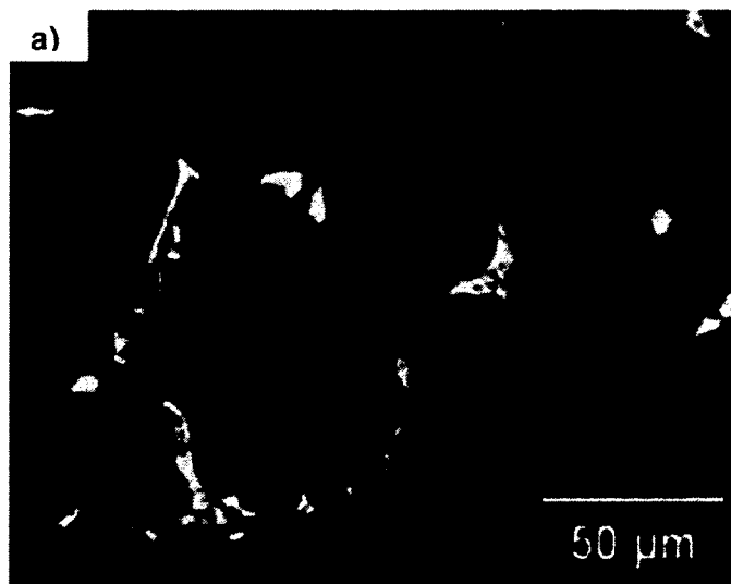
Figure 4.5: a) SEM micrograph of the as-cast B206 test sample after the immersion corrosion test
