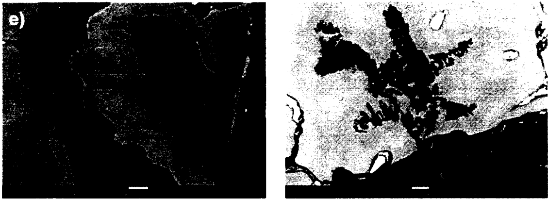
Figure 4.4: e) & f) SEM micrographs of the as-cast B206 test sample after the immersion corrosion test.
