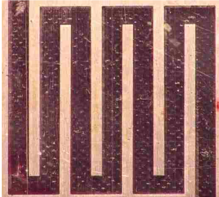
(b) t = 0.13 s; Liquid water accumulated at the bending area of the first segment in the channel
