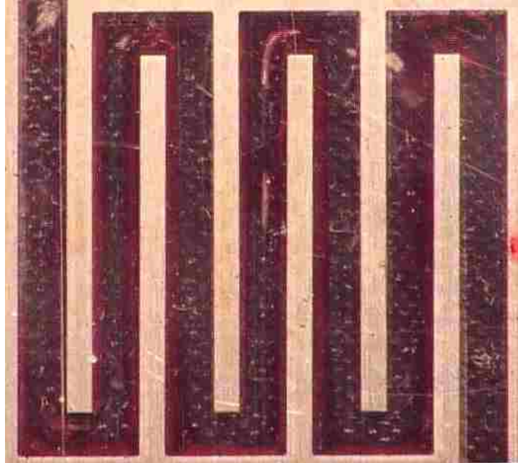
(d) A thicker area at the head of the liquid water slot observed when the slot reaches the bending area of the channel
