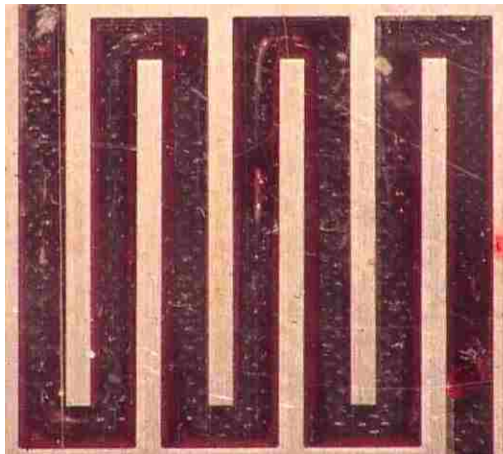
(e) t = 1 s; The liquid water slot approaching the outlet of the channel
