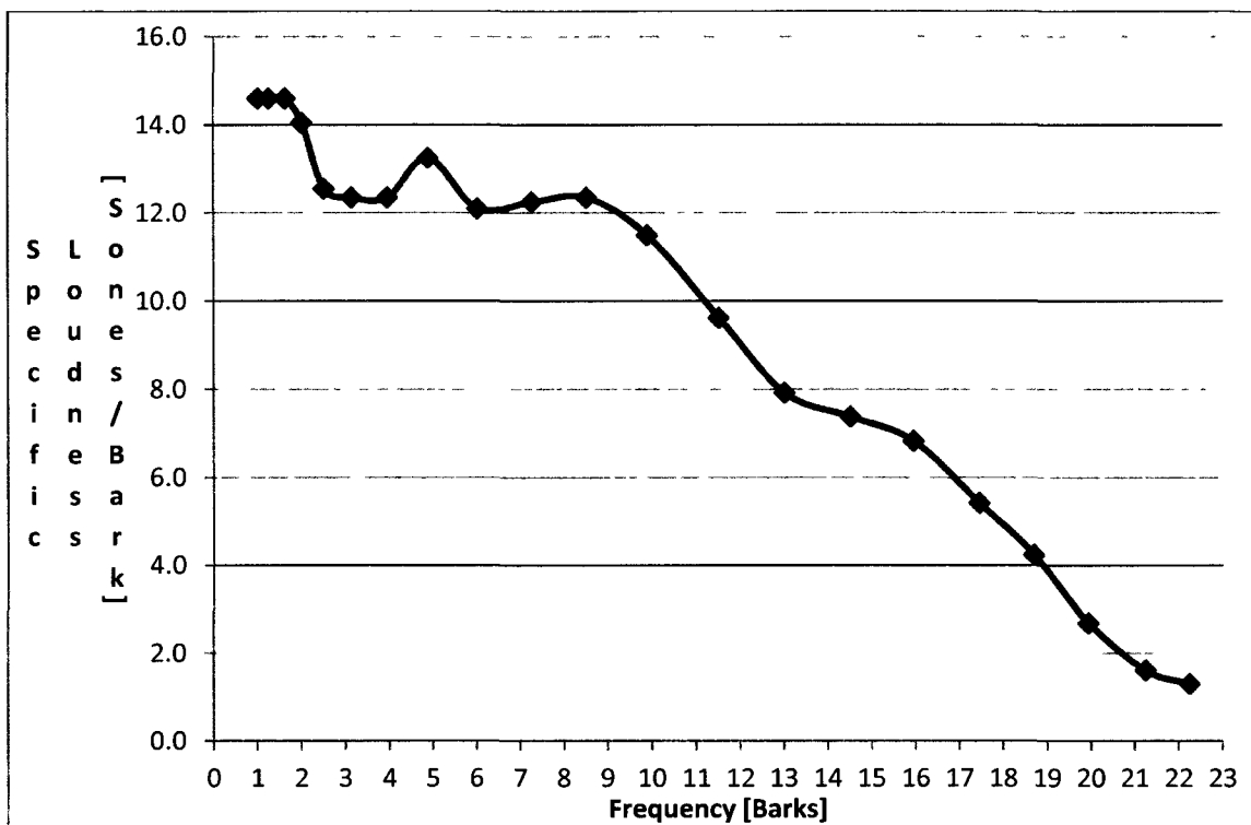
Figure 81: Averaged Specific Loudness for a Diffuse Field Sound Field Condition from Microphones 1 and 5 for the 4.7 mm Thick, 60cmX60cm Sample of 6061-T6 Aluminum, Demonstrating Irrelevancy, for Periodic Random or Scattered White or Pseudorandom Noise 10 Seconds Signal Duration, 106.9 dB in the Reverberation Pit
