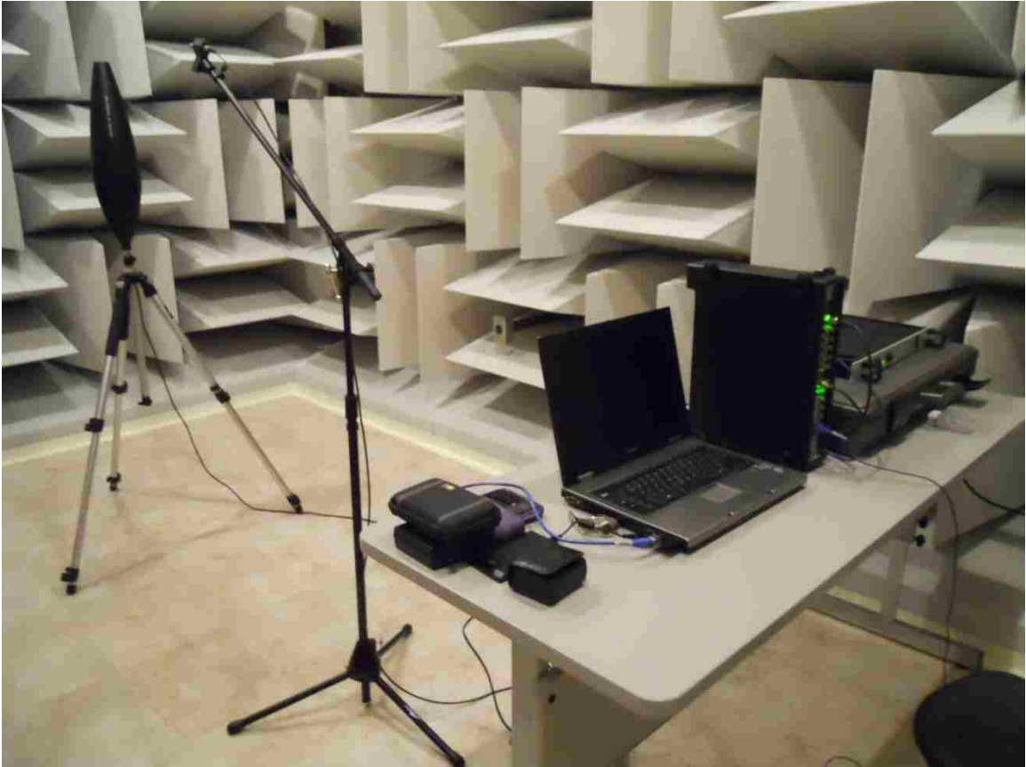
Figure 18: Photograph of the experimental set up in the Semi-Anechoic room showing the Bruel & Kjaer acquisition system, amplifier loudspeaker and microphone. The test sounds are generated by the PULSE sound generator and played by the loudspeaker and subsequently recorded through the microphone. The acquisition system then prepares the WAV file for the multiple look gap correction and loudness programs.
