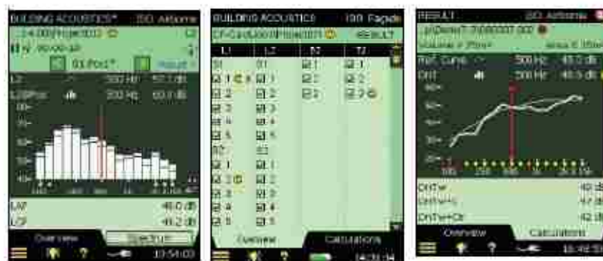
Fig. 24: Examples of building acoustic measurements using Type 2259/2270 L2 average and L2 at one position (Left), Overview of measurements (Center), Final result (Right)
