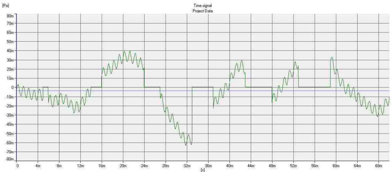
Exhibit C2 - 60 dB Steady Sinusoidal Test Signal with Gaps
