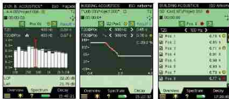
Fig. 22 Reverberation time spectrum (left), Reverberation decay curve (centre), and Overview of results (right)
