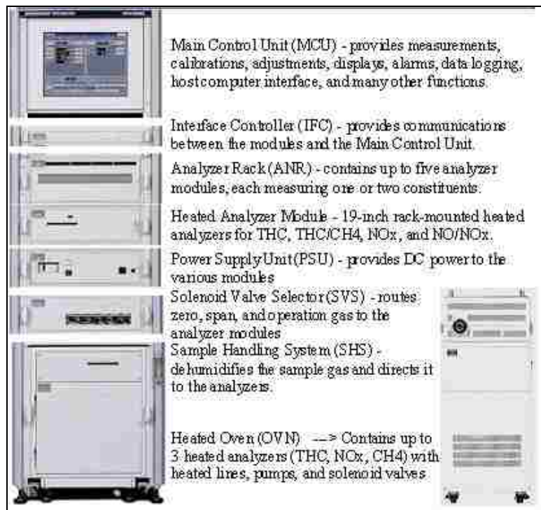
Figure 3.5: HORIBA MEXA-7500 Emission Analyzer System [13]
