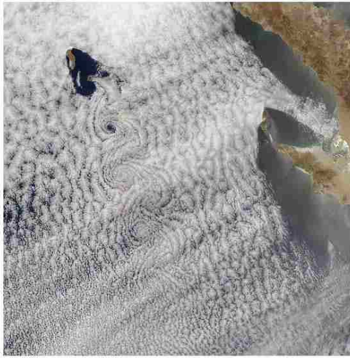
(a) Type A Instability: Oceanic wake at Guadalupe Island, California (Reproduced according to the general terms of use, NASA Visible Earth Repository).
