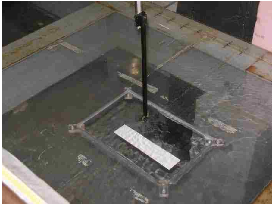
Figure 3.1: A picture of the bluff body used in the experiment.
