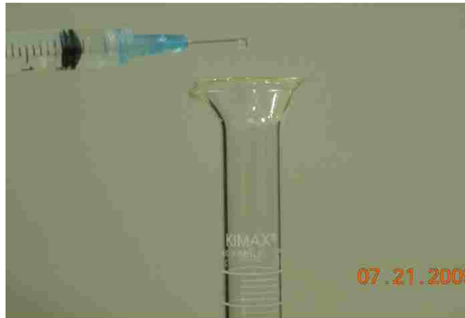
Figure 7.3: Description of creating the droplets
