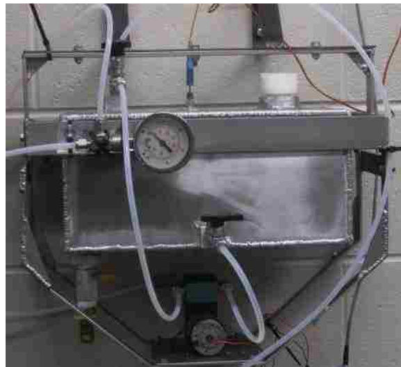
Figure 4.11: Water Cooling System
