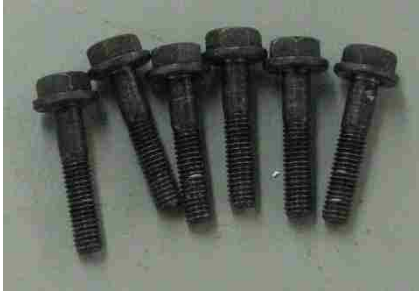
Figure B.16: M6 Flange Bolts
