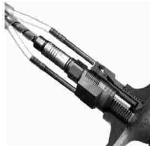
Figure 4.9: Kistler Pressure Transducer Assembly (Taken from [19])
