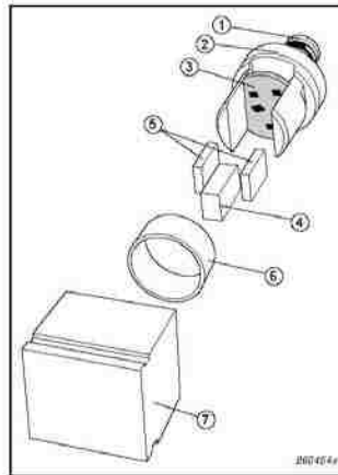
Fig. 1 Exploded view of Miniature DeltaTron Accelerometer Type 4508 (top mounted connector) showing the ThetaShear design and the built-in DeltaTron preamplifier
