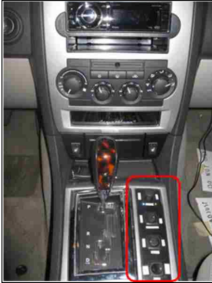
Figure 4.4 – Custom Made Switchboard to Switch between Subwoofer Systems
