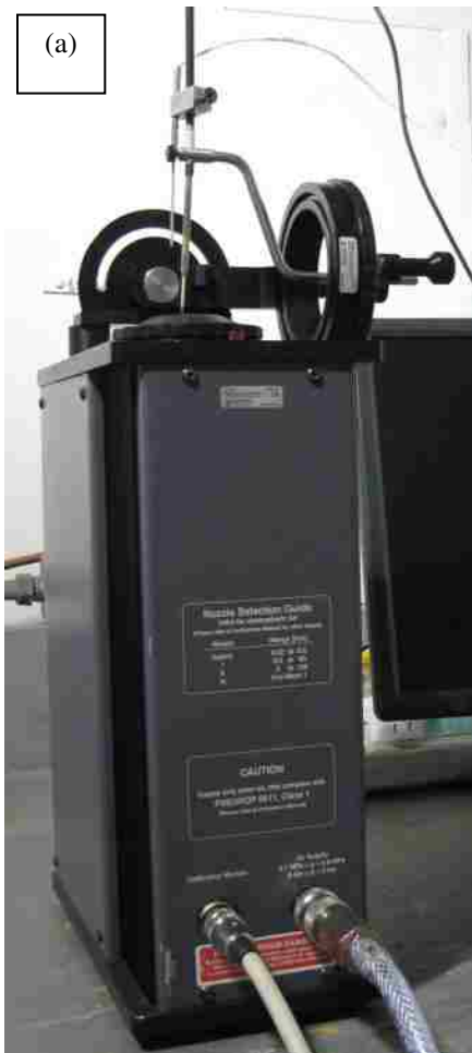
Fig. 22 Hot-wire calibration system (a) calibration unit, and (b) air supplier
