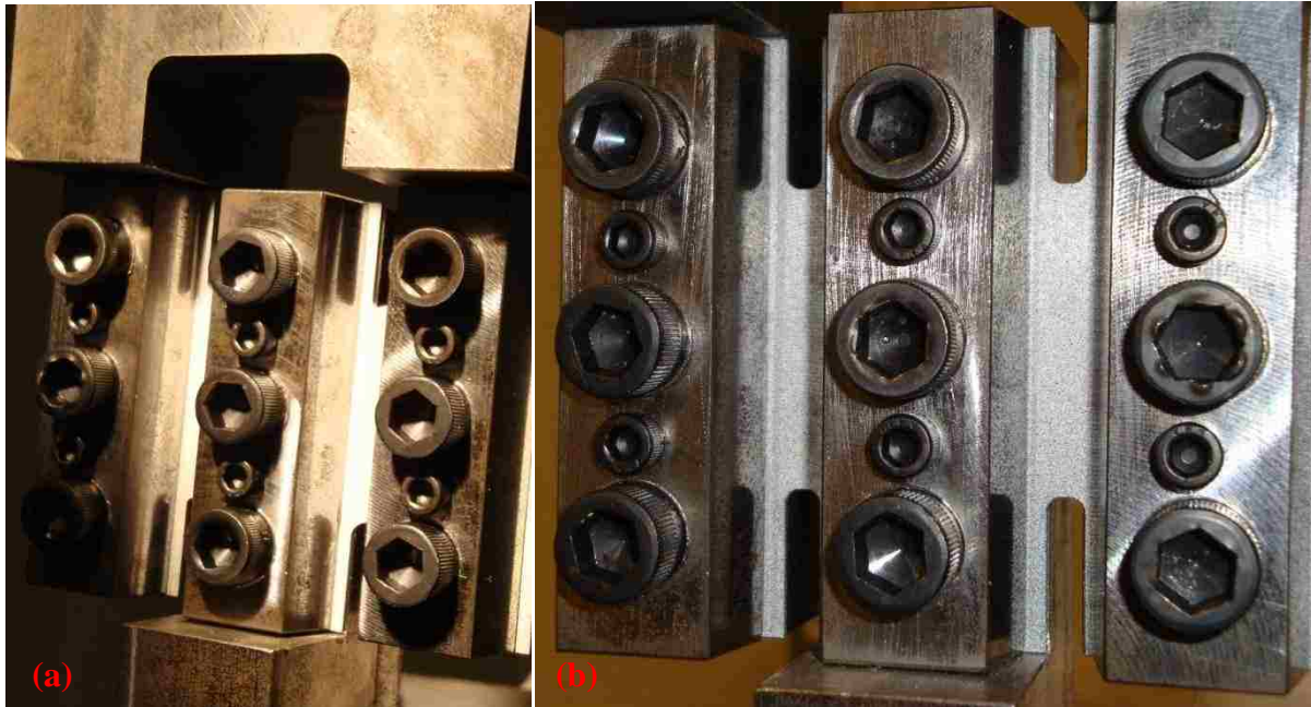
Figure 4.8 Cyclic shear test (a) specimen set up between fixed upper and lower movable fixture (b) specimen and two shearing gauge zones of the specimen
