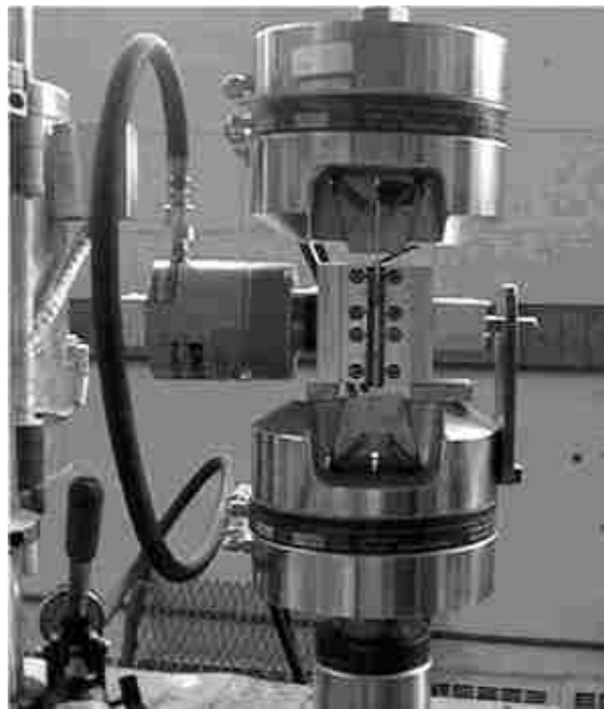
Figure 2.17 Schematic of the cyclic tension-compression device developed by Boger et al. [91]
