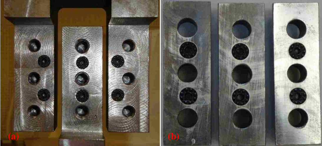
Figure 3.15 Photograph of inserted knurled blocks on the surfaces of (a) the upper and lower fixtures, and (b) the holding blocks of the cyclic shear test fixture
