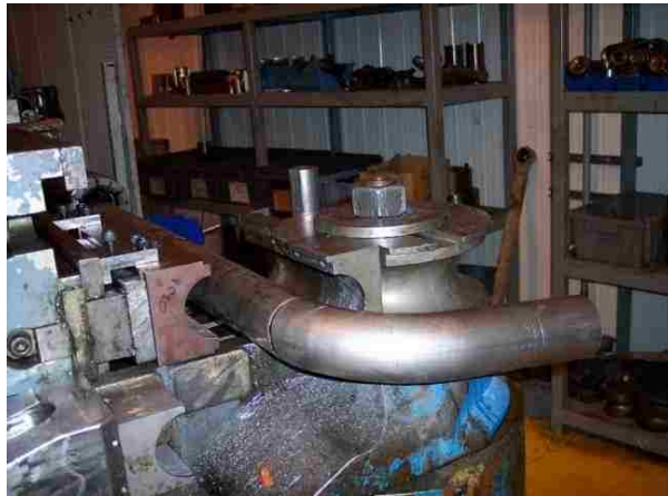
Figure 2.18: Example of a steel tube which has undergone rotary draw mandrel bending
