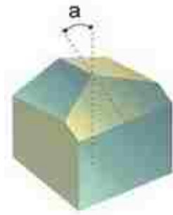
Figure 2.25: Ideal Berkovich indenter ( a = 65.35^\circ )
