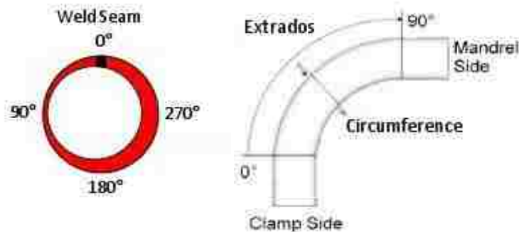
Figure 4.2: Orientations and angles used for strain measurements
