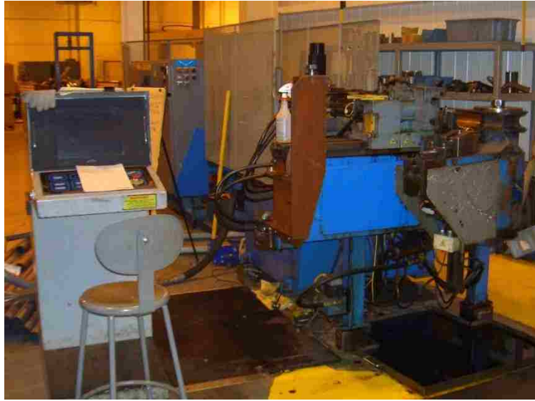
Figure 3.4: Eagle Precision Technologies rotary draw mandrel bender
