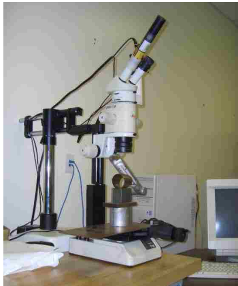
Figure 3.6: Circle grid strain measurement equipment
