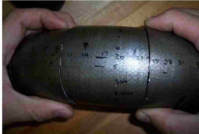
Figure 3.5: Circle gridded section on a bent tube
