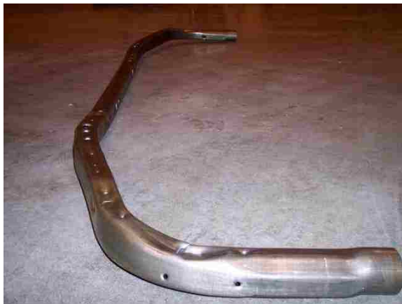
Figure 2.20: Example of an upper fender rail produced by hydroforming
