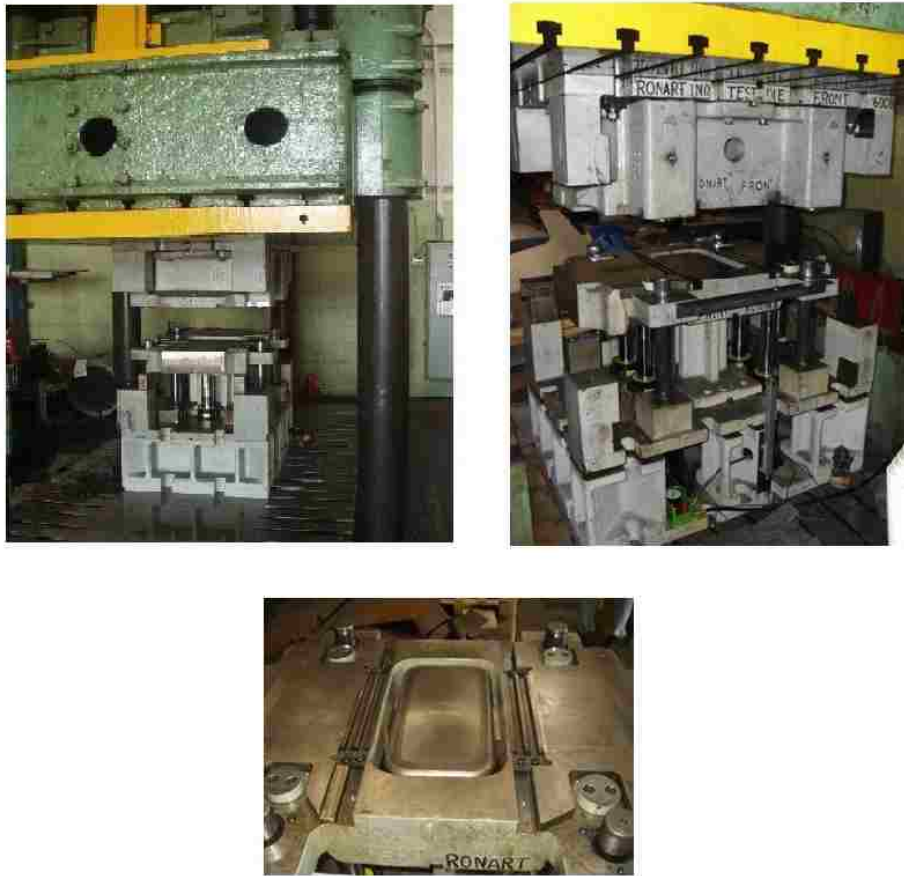
Figure 3.1: A/SP die installed in a hydraulic press
