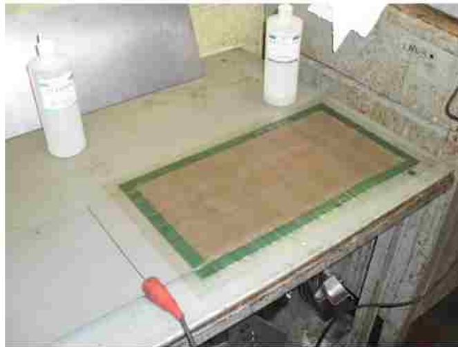
Figure 3.7: Electroetching a grid of circles of 0.1(in) diameter onto one side of a blank
