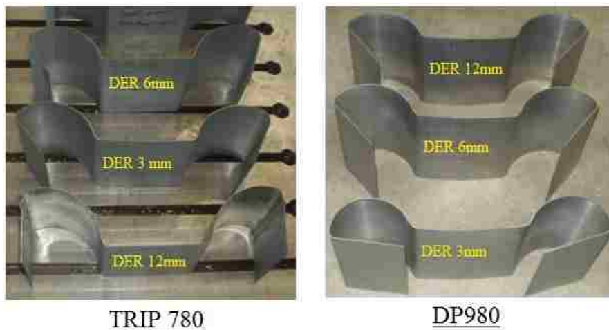
Figure 3.14: Channels drawn with various die entry radii and without drawbeads
