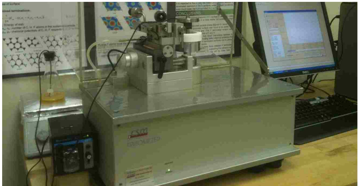
Figure 3- 4: Setup used for pin on disk wear tests.
