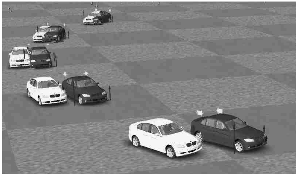
Figure 7.3: Case 1: open-loop step steer input response, visualization. This figure presents the response of the uncontrolled and controlled vehicle to an open-loop 50^\circ step steering wheel input. It can be seen that the applied yaw moment across the rear axle of the controlled vehicle (black) improves cornering response without additional driver steer input.
