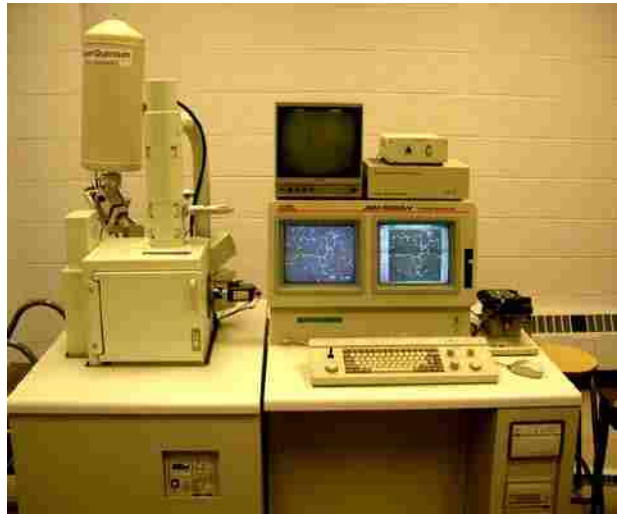
Figure 3-8 Scanning electron microscope (JEOL Model JSM-5800 LV).
