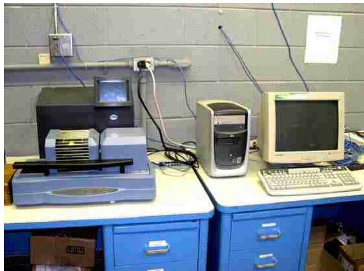
Figure 3-9 A differential scanning calorimetry-thermogravimetric analyzer (DSC-TGA Q600).
