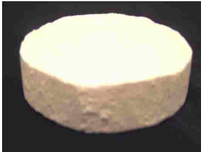
Figure 4-1 A hybrid preform made from the \text{Al}_2\text{O}_3 particles (4vol %) and fibres (9vol %).
