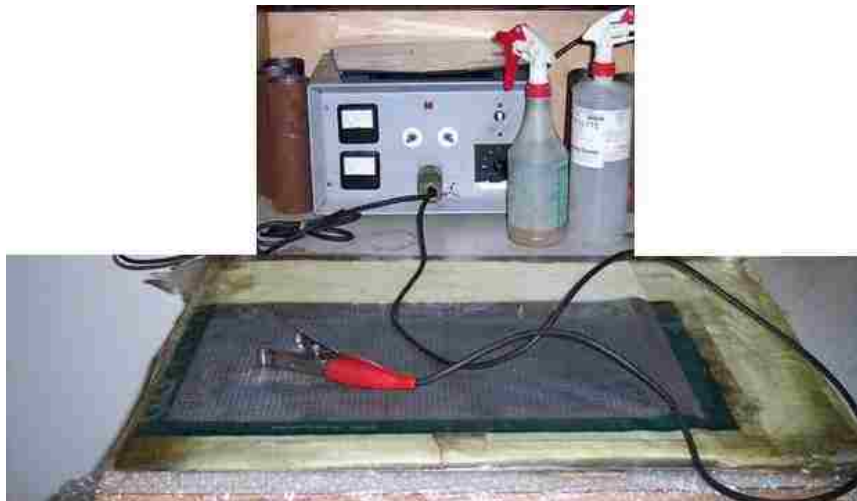
Figure 25: Electro-etching apparatus and grid pattern sheet
