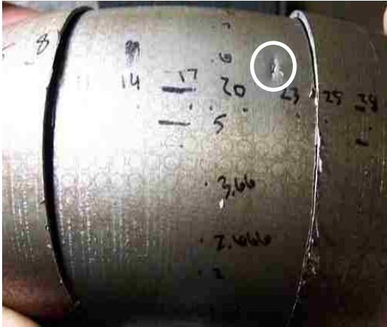
Figure 43: Surface crack on a bent tube
