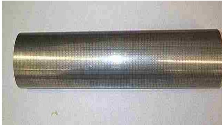
Figure 24: A tube electro-etched with circle grids
