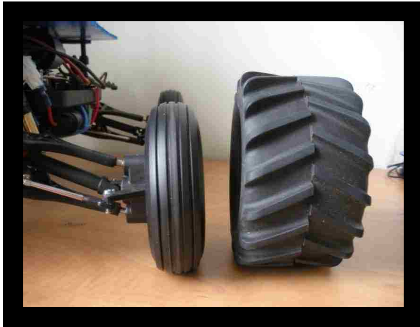
Figure 11: Du-Bro tire vs stock E-Maxx tire comparison
