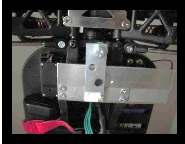
Figure 51: Steering potentiometer mounting
