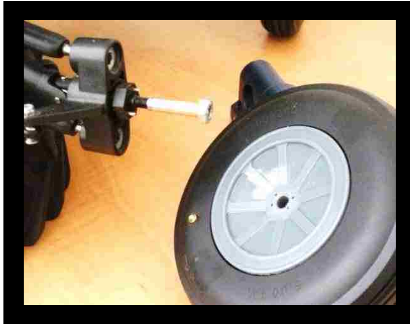
Figure 12: Modified E-Maxx wheel assembly
