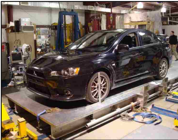
Figure 15: VIMF Testing This testing was carried out courtesy of SAE Ltd at the Columbus, Ohio facility.
