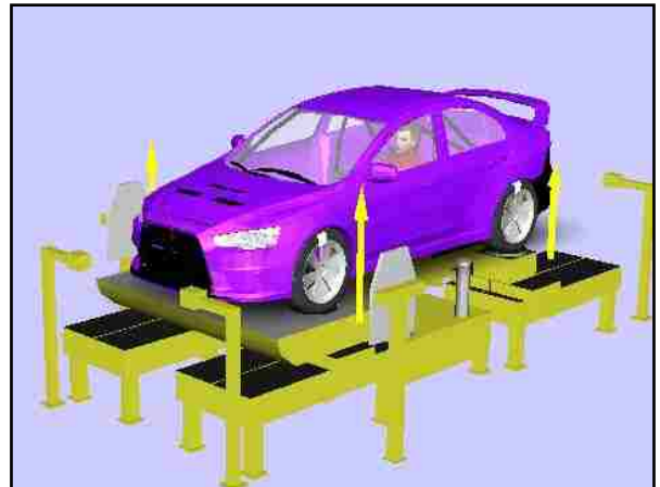
Figure 16: CarSim Model Screenshot of the CarSim digital model, in place on the virtual shaker rig.
