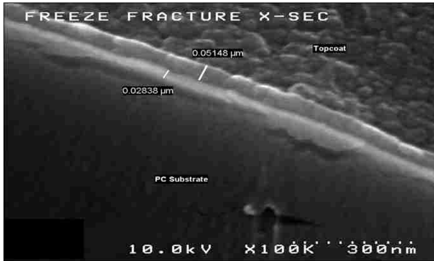
Figure 6.3: SEM Images for Freeze Fracture of a Cross Section for a Typical Sample for System-B
