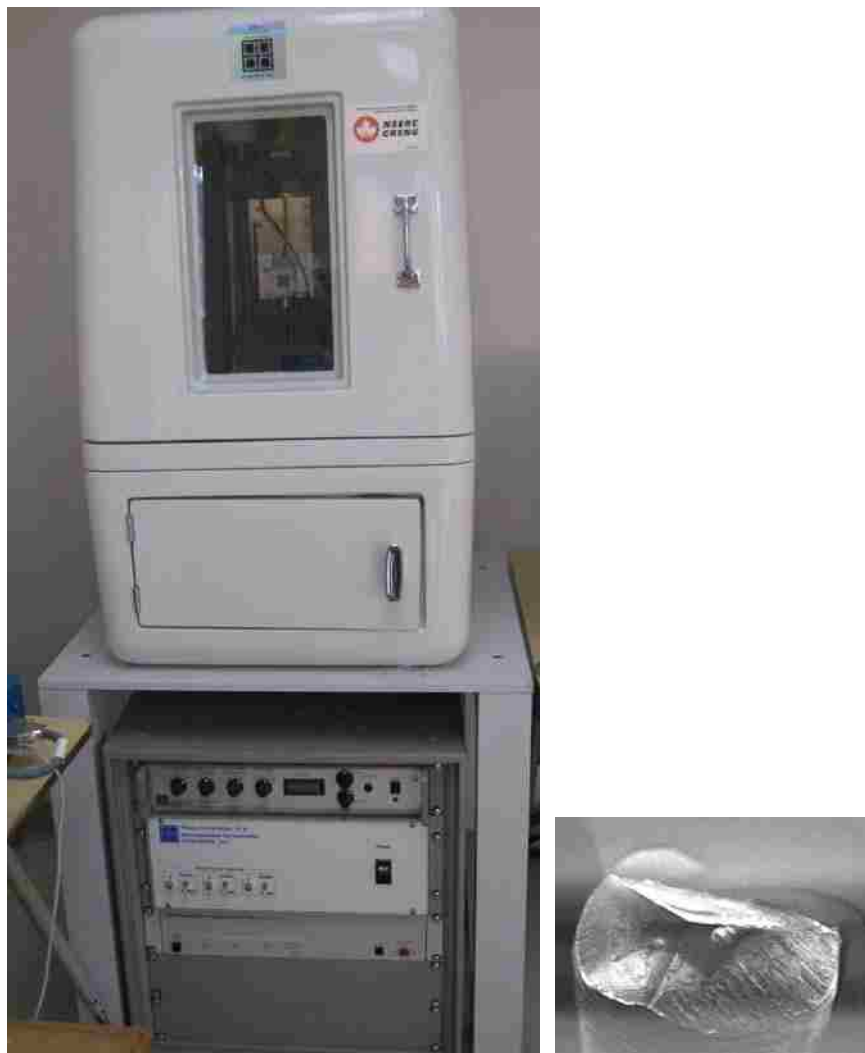
Fig. 3.9 Ubi 1 TM nano-mechanical testing system and Berkovich tip used in hardness test.
