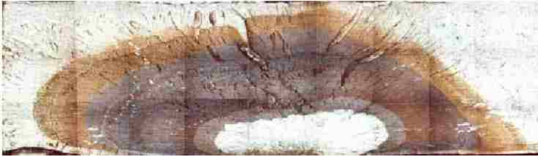
Fig. 2.7 Through-wall crack in a CANDU Zr-2.5Nb pressure tube, showing oxidized crack growth bands. The crack initiated at the inside surface just inboard of the rolled joint [37].
