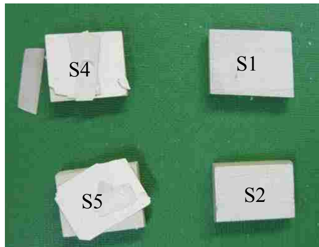
Fig. 4.20 Photos showing the spalled-off oxide from PEO coated samples of Group B after 30-day autoclave treatment.
