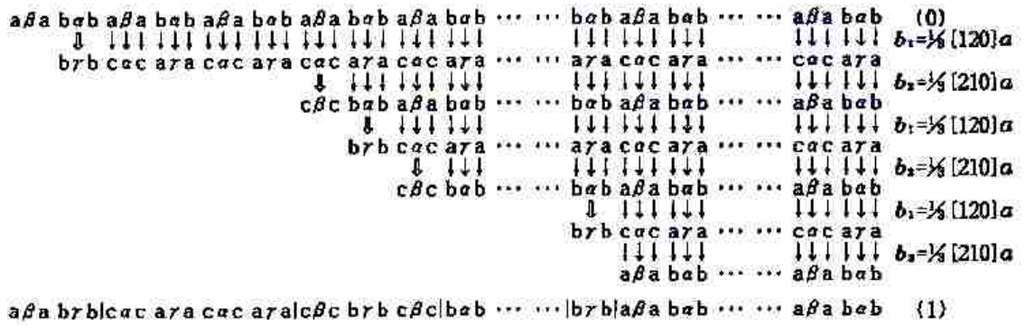
Figure 8 Formation mechanism from an original perfect hexagonal WS 2 crystal (0) to the structure (1) in the lowest part of the crystal: ↓, atoms shifts by slipping between S-S layers; || local shifts of W atoms. b 1 and b 2 are glide vectors, which are partial in the complete Burger vector b=a[110].
