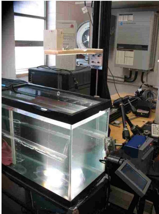
Figure 3.2: Picture of experimental equipment for spheres falling from rest.
