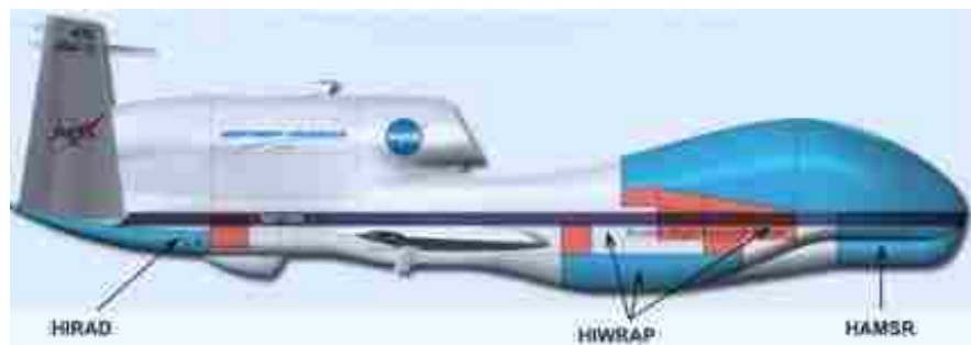
Figure 2-1: Global Hawk UAV with major remote sensor instruments.
