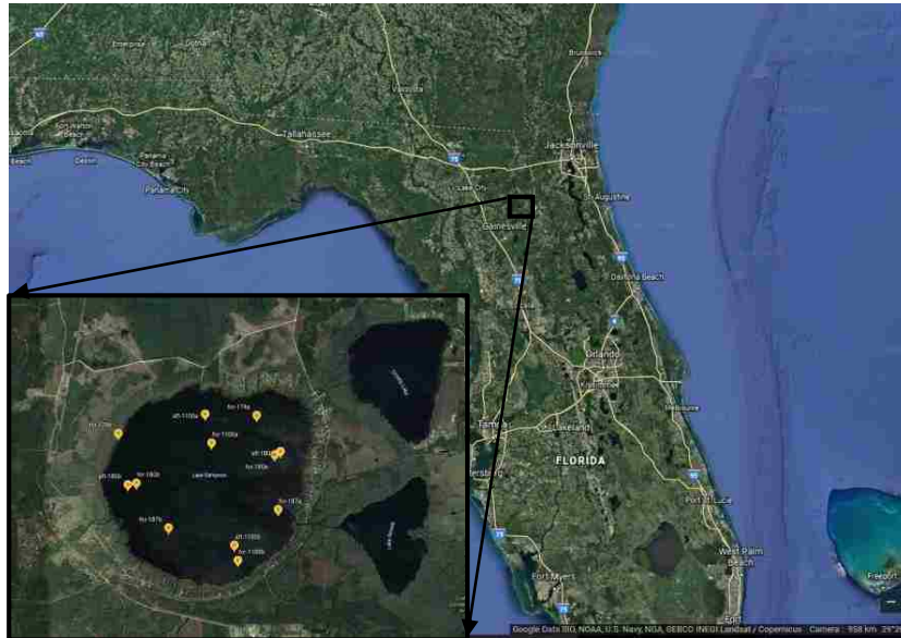
Figure 3-12: HIWRAP geolocation analysis for Lake Sampson. Yellow markers are the location of the maximum reflectivity slopes.
