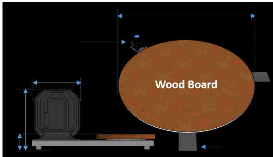
Figure 4.3: Footstep platform: We placed a round wooden board on top of three floor plates. For added stability we added rubber support bumpers between each plate at the boundary. A low frequency audio transducer was mounted at one of the floor plates. Participants stood in the center of the platform during the experiment.
