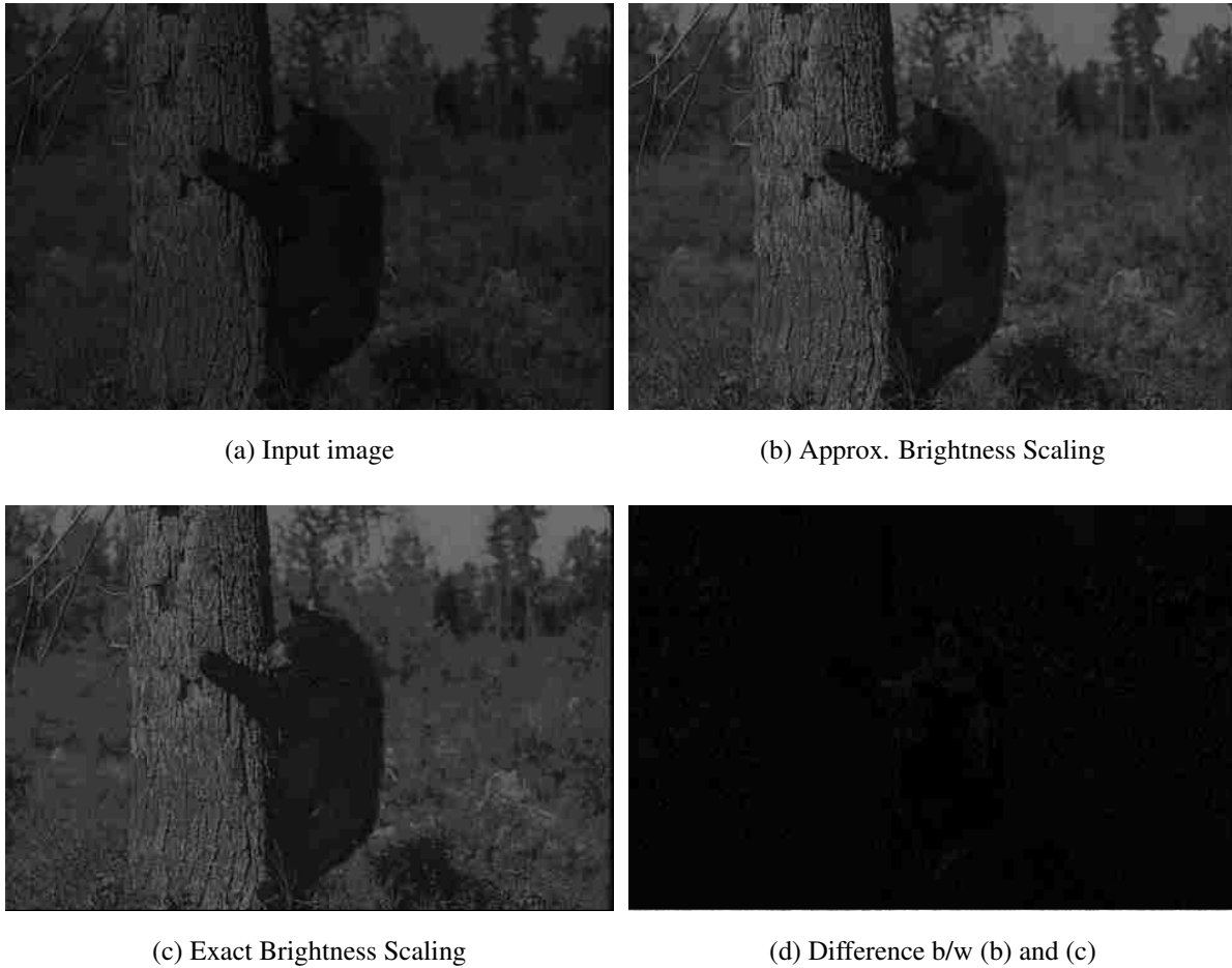
Figure 6.10: Performance of our approximate circuit for brightness scaling. (a) is the original image, (b) shows the result of 60% scaling with our approximate kernel, (c) is image after 60% scaling with exact kernel, (d) is the difference between the two results. Our approximate design was 46% more compact than the exact counterpart
