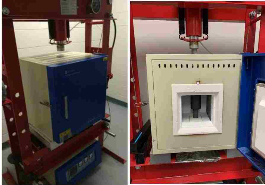
Figure 22. Photos of the hot-press with oxygen gas supply line in the back side of the furnace.
