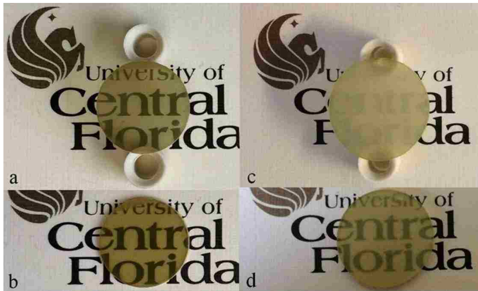
Figure 33. Photographs of PMN-PT ceramics made from (a&b) combustion-synthesized lead oxide; (c&d) and from commercial lead oxide.
