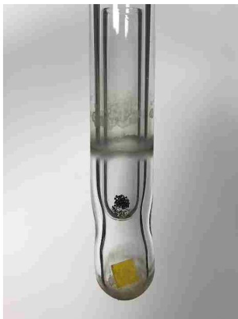
Figure 48. Quartz ampoule used in the experiment.
