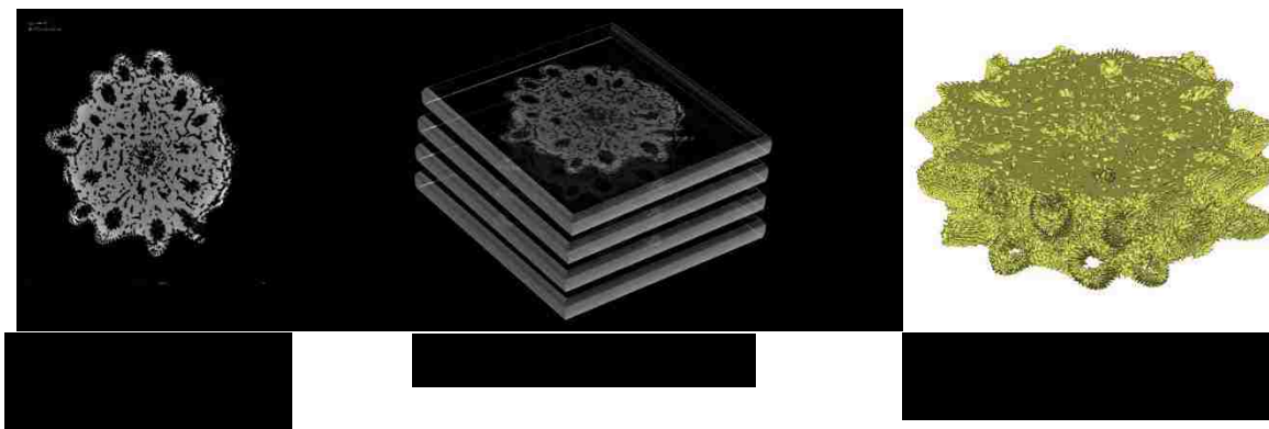
Figure 47: Steps involved in the generation of the 3D computer-aided model of the coral skeleton from the images provided by the CT scan video.
