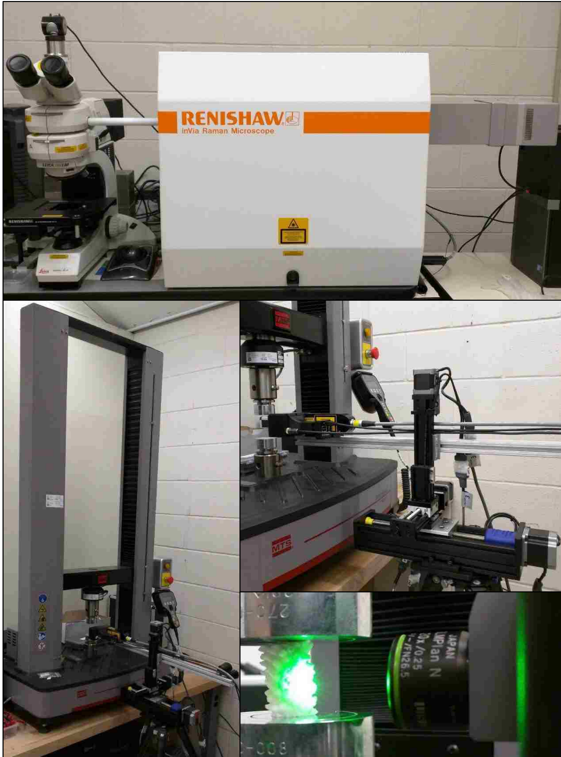
Figure 52: Components used for the development of the Raman spectroscopic probe for in-situ analysis of ceramic materials.
