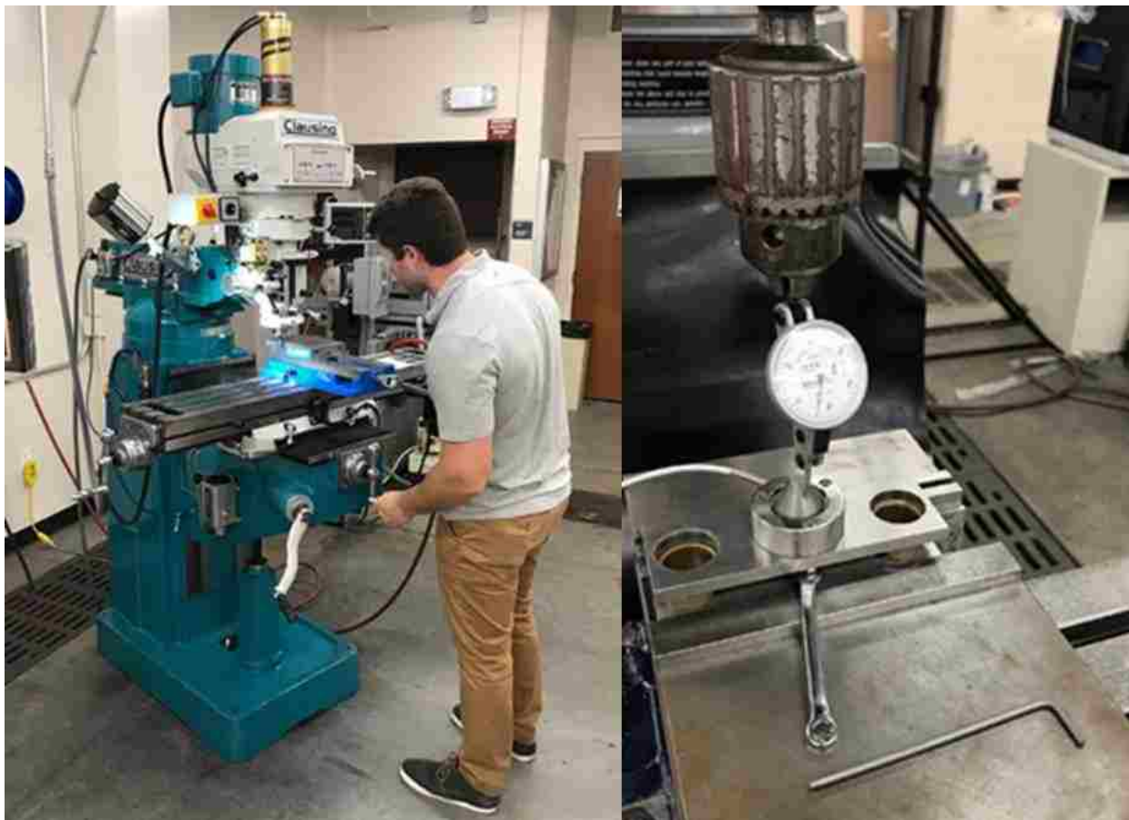
Figure 50: UCF machine shop vertical mill (left) and load cell alignment (right).
