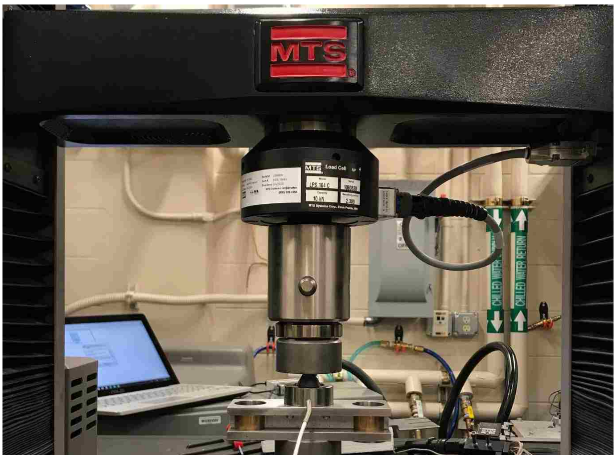
Figure 56: Load Cell Calibration using MTS Criterion Model 43 universal testing machine.
