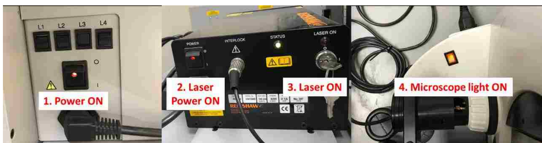
Figure 62: Raman spectrograph machine power on procedure.
