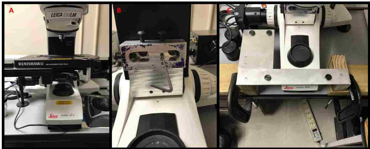
Figure 61: Compression stage setup. A) two-axis mapping stage, B) mounting fixture, C) elevations system.
