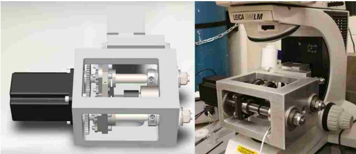
Figure 24: First compression stage designed produced by UCF senior design team.
