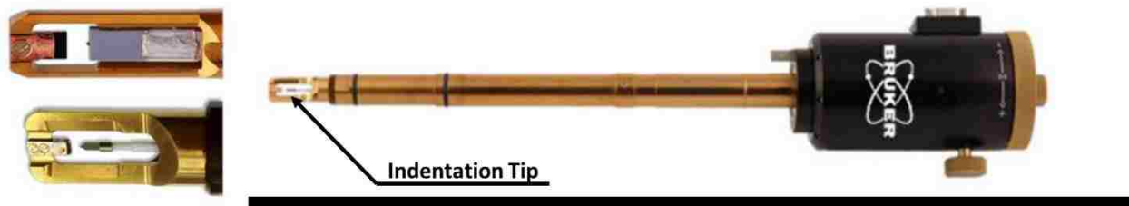
Figure 10: Hysteron PI 95 TEM Pico indenter with close of loading tip [22].
