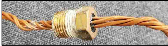
Figure 4-8 Thermocouple feedthrough used in evaporator/condenser chamber
