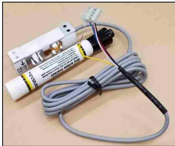
Figure 4-3 Pictorial view of the load cell used in this study
