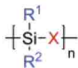
Figure 2 Generalized representation of the molecular structure of pre-ceramic organo-silicon PDCs precursors. 2
