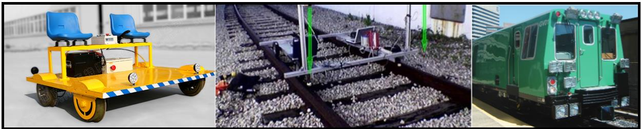
Figure 1 Various platforms for railroad inspection
