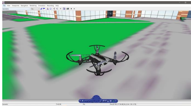
Figure 10 3D Simulation of Parrot Mambo mini drone flight using MATLAB/Simulink.
