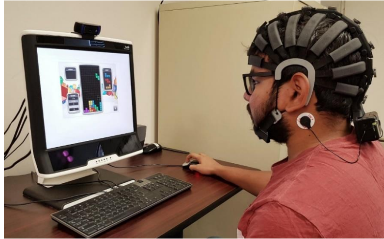
Figure 4.3. A Subject Wearing 64-Channel EEG Device During the Experiment
