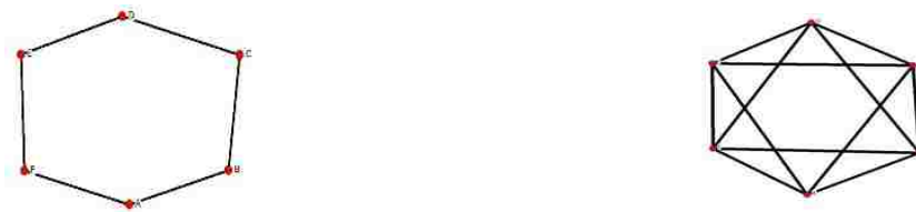
a. 2-regular graph with n = 6, k = 2, M = 3 b. 4-regular graph with n = 6, k = 4, M = 12
