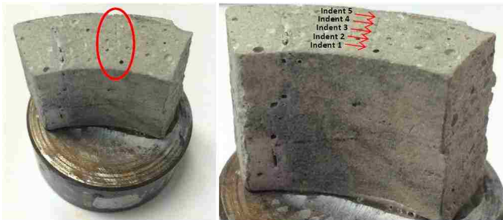
Figure 4.7: Indentation points of the cement sample. Indents range from the inner pipe side of the sample (Indent 1) to the outer pipe side of the sample (Indent 5).
