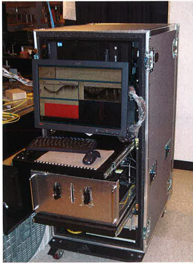
Figure 3.5 – Multifunctional Optical Coherence Tomography System showing separate displays allowing for continuous real time updates of spectrum, intensity, flow and polarisation properties of the sample being imaged.
