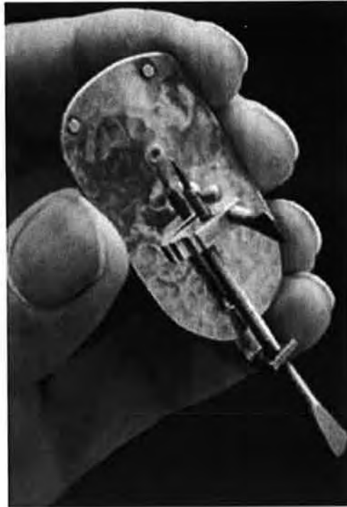
Figure 2.3 - An example of a microscope as designed by Antoni van Leeuwenhoek. The sample is placed on the pin and brought into focus using the screw. This image is of a replica built by Al Shinn (Shinn).
