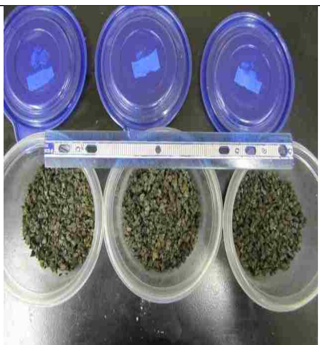
Figure A.11: CO 2 -brine flooded crushed shale samples after three months
