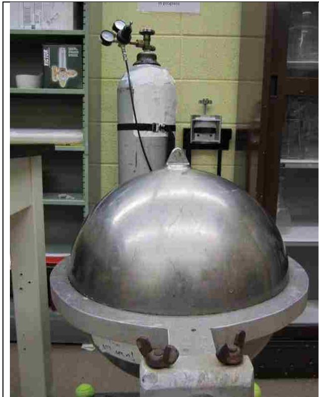
Figure A.6: CO 2 -brine preparation setup showing CO 2 cylinder and mixing tank
