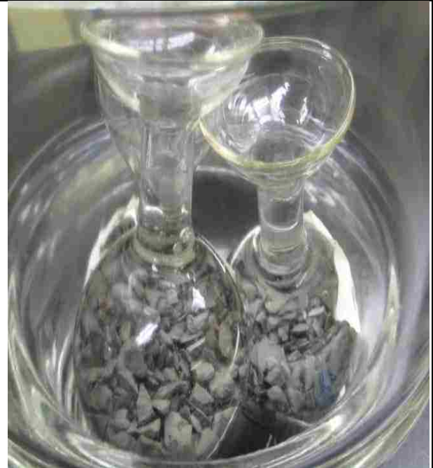
Figure A.5: Crushed shale caprock control sample re-saturation under vacuum condition
