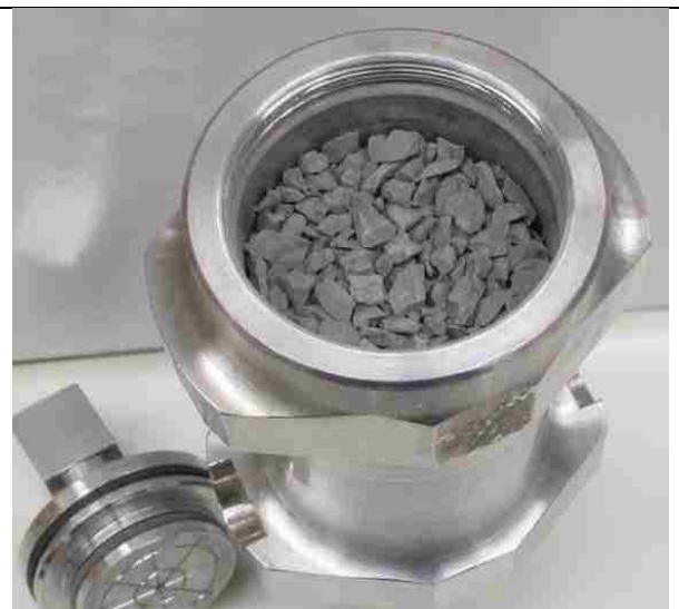
Figure A.3: Crushed shale caprock sample packed into a pressure cell
