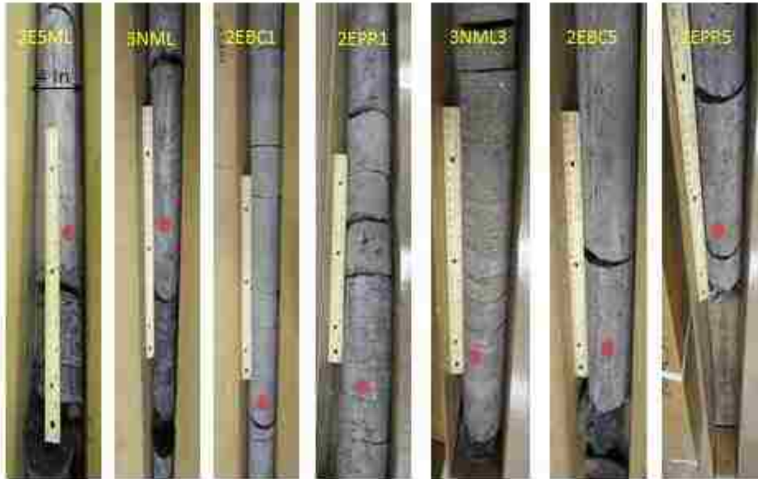
Figure 3.4: Physical shale caprock cores from the Pottsville Formation, Alabama
