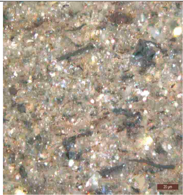
Figure E. 8: Optical Microscopy image of thin section cut for control sample A showing pore networks
