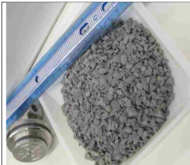
Figure A.2: Crushed shale caprock samples showing particle dimension
