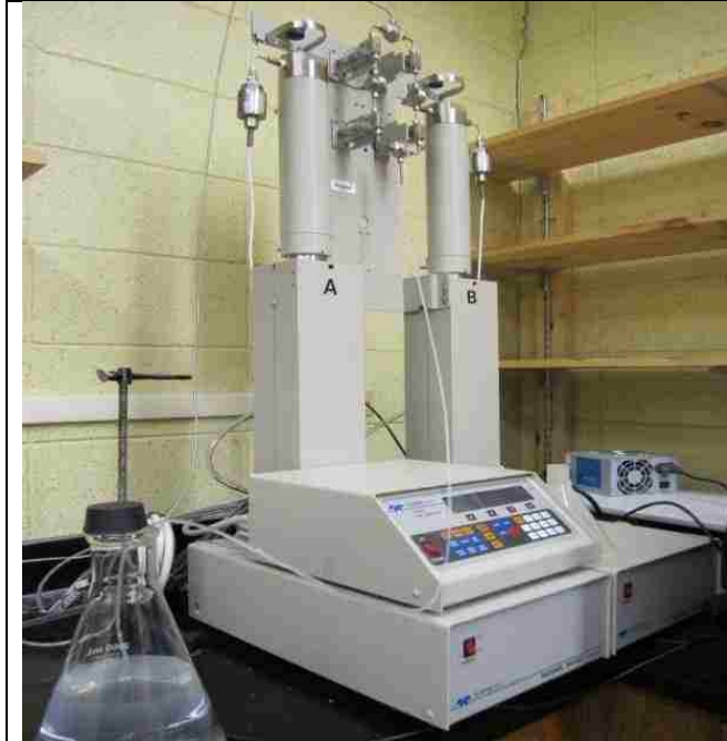
Figure A.4: Syringe pump used as backup pump in shale caprock/CO 2 -brine flooding
