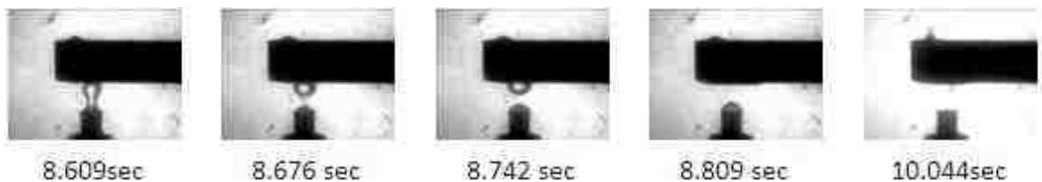
Figure 50: Dynamic Behavior of Condensate Drop on Lower Surface A after 1500 ppm Anionic Surfactant Injection at 2264 psia and 210 °F
