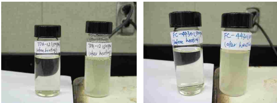
Figure 11: Phase Behavior Pictures for 500 ppm Nonionic Surfactants TDA-12 and FC-4430 Solutions at 72 °F and 210 °F
