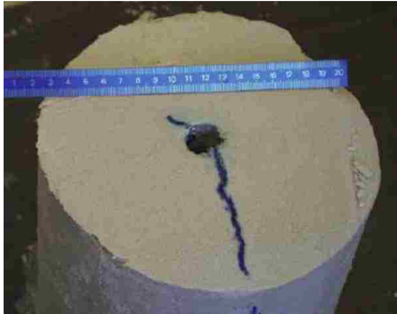
Figure 3.2. Fractures obtained with cross linked gel plus quartz powder (Bohloli, 2006)
