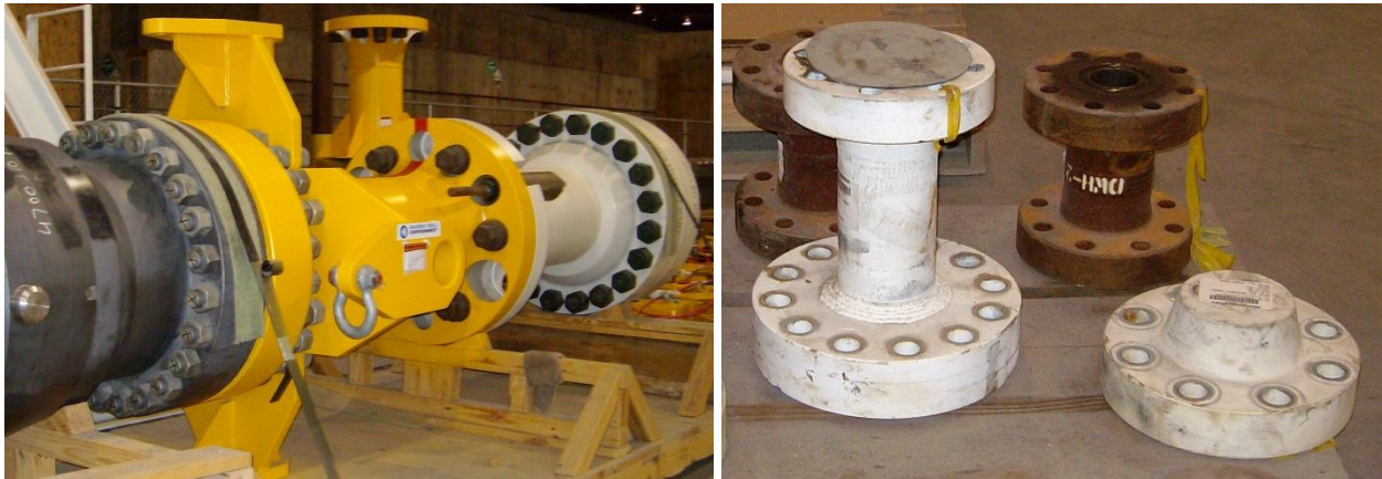
Figure 13. Well containment warehouses are being stocked so emergency responders can react to blowouts with the right equipment in a timely fashion. Depending on the function and pressure rating, flanges may have a few thick bolts or several of them evenly spaced out. Photographs were taken by Muhammad Zulqarnain while on tour at the Marine Well Containment Company’s facility in Houston, Texas.
