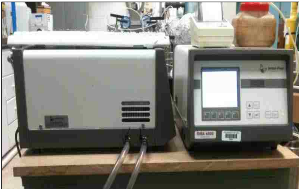
Figure 20: A picture of the DMA HP density meter connected to the DMA 4500 evaluation unit
