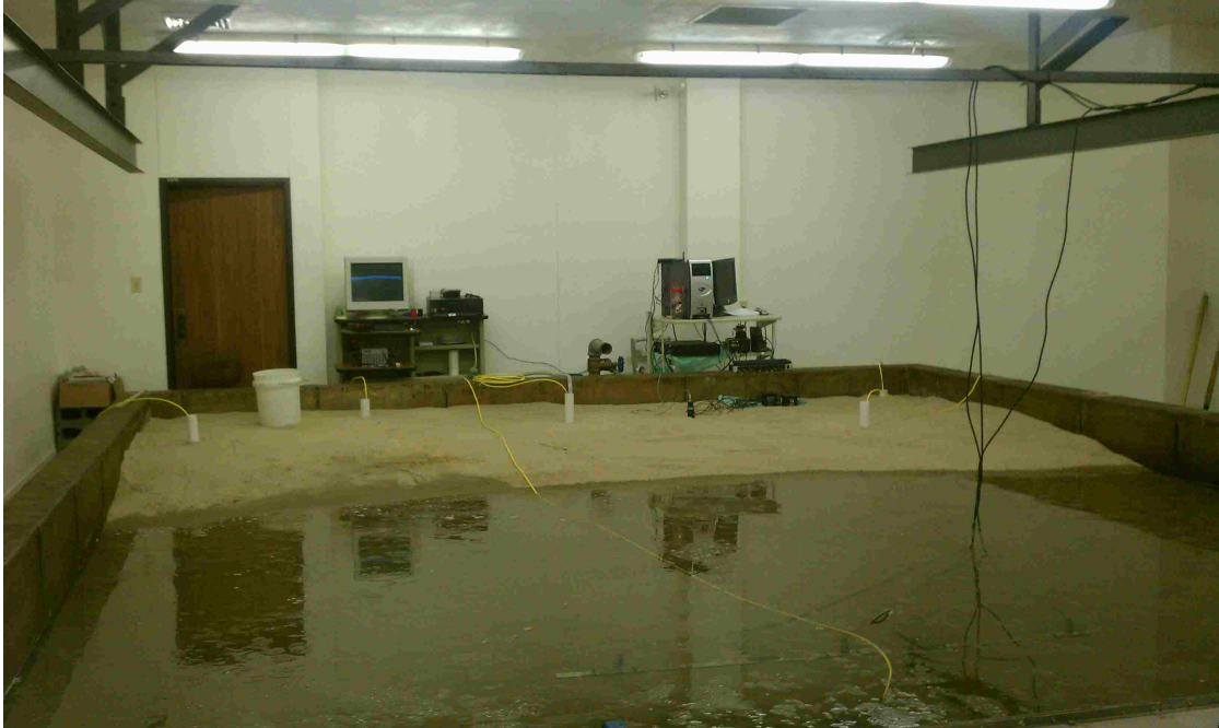
Figure 4.3: Sand tank data acquisition setup. The figure shows all five monitoring wells with PT sensors and all seismic data collection equipment ready to collect data. This is the equipment configuration used to collect observations for this thesis. Also, notice the capillary forces absorbing water up into the formation above the water line at the free water end of the tank.
