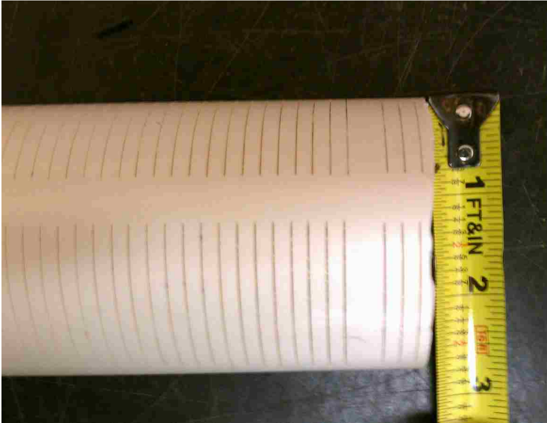
Figure 5.4: Slotted PVC used for wells in sand tank. Pictured above is the 2" circumslotted, ten slot (ten slots per inch), PVC pipe used in the construction of the wells within the sand tank. The slot size is 0.010", or 0.000254 m. These slots act as perforations in the well bores of the sand tank. There is no production tubing inside the production wells, the well produces straight through the casing.
