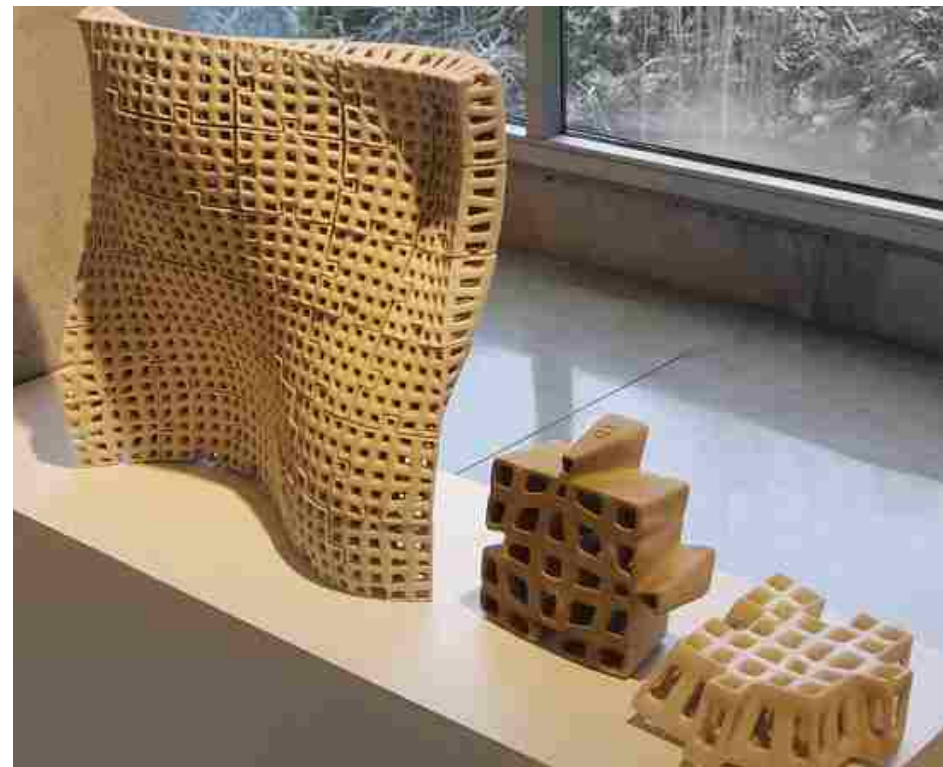
Figure 29: 3D printed bricks, http://www.news.cornell.edu/stories/2014/07/3-d-printing-helps-designers-build-better-brick .
