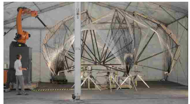
fig. 24 Continuous fabrication of fiber shell
