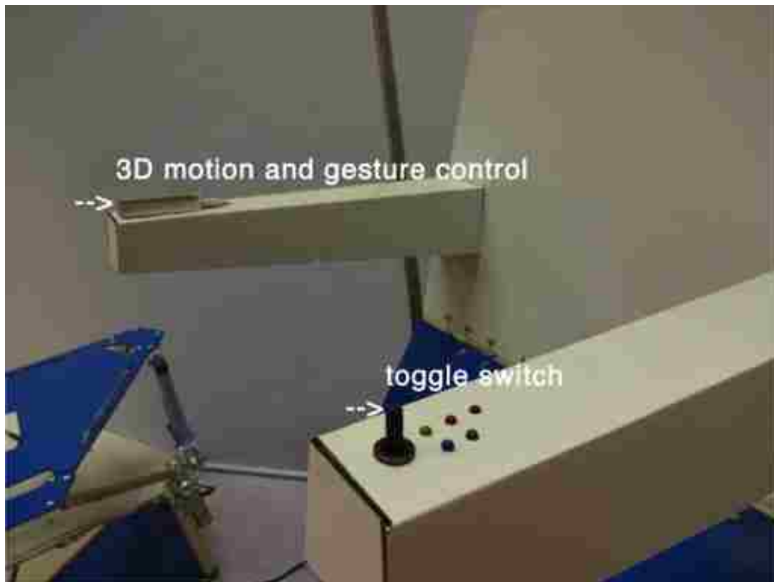
Figure 43 - Controls on the chair's armrest
