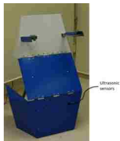
Figure 42 - Chair's ultrasonic sensors
