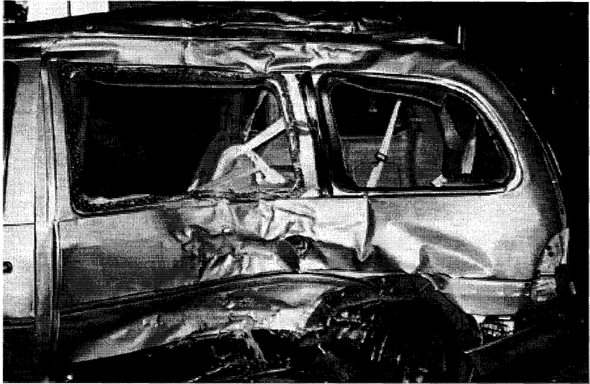
Figure 12. Side impact with a tree, Case 9 [55].
