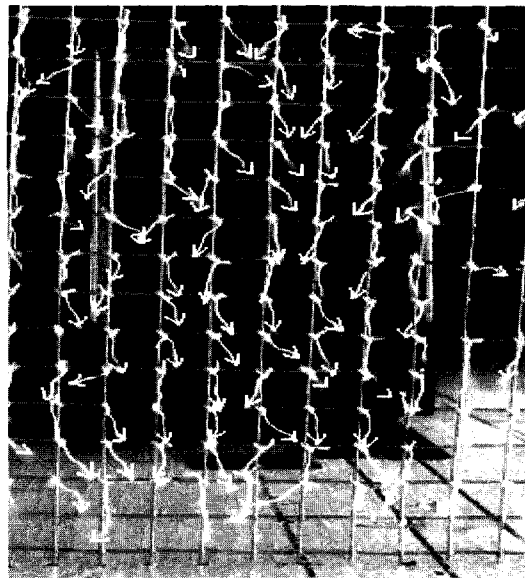
Figure 4.29 Tuft visualization: X=1.5H downstream, 14m/s freestream
