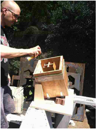
6. applying release agent : PAM
