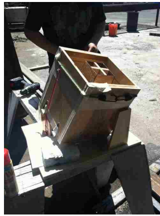
8. tilted mold assembly
