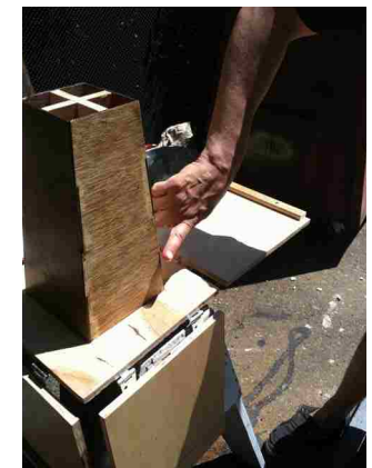
5. applying release agent : vaseline
